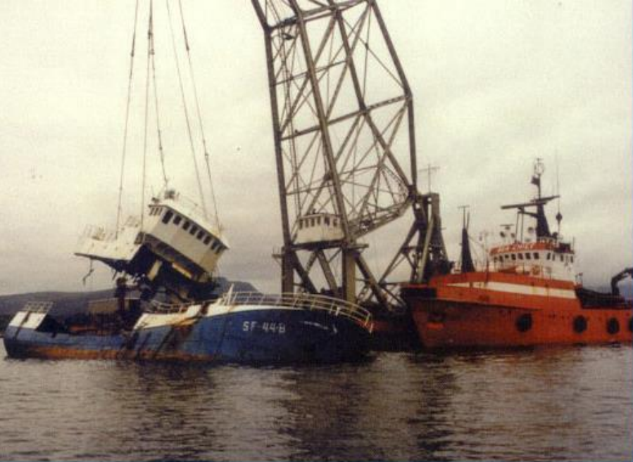
Wreck removal of M/V «Oldersund» with a steelweight of 240 tonn from 10 m. at Rørvik January 1997.
