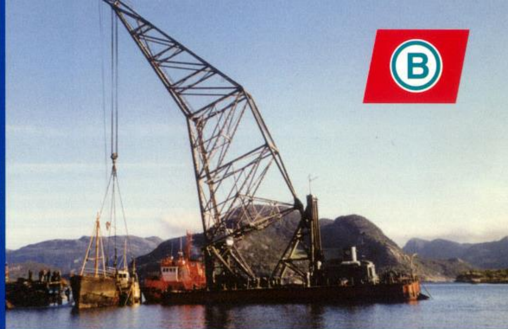
Wreck removal of M/V «Oldersund» with a steelweight of 240 tonn from 10 m. at Rørvik January 1997.
