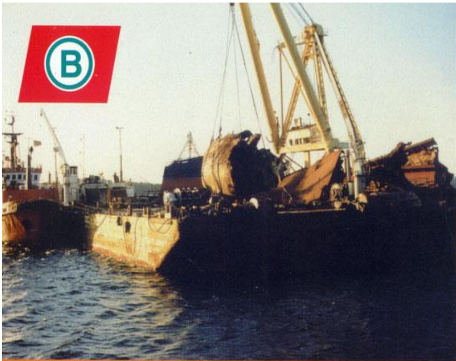
Wreck removal of M/V «Sønnodd» with a steelweight of 550 tonn from 17 m. at Grimstad summer 1999.
